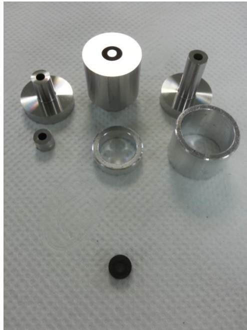
Figure 2.5 Toroidal shaped pellets and dye components.
