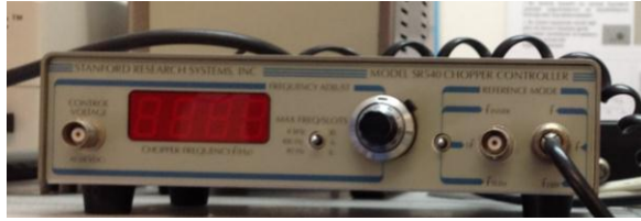
Figure 2.4 The chopper used for our study (Stanford Research Systems SR540)
