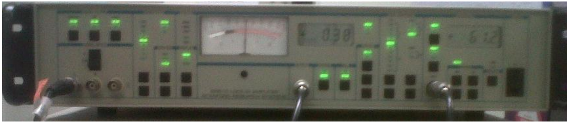
Figure 2.7 The lock-in amplifier used in our study (Stanford Research Systems, SR510)
