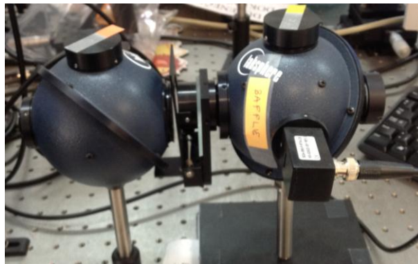
Figure 2.5: The Double Integrating Sphere System at Boğaziçi University, Institute of Biomedical Engineering (Labsphere General Purpose sphere, spectralon, 4 ports-0.33 inch diameter)
