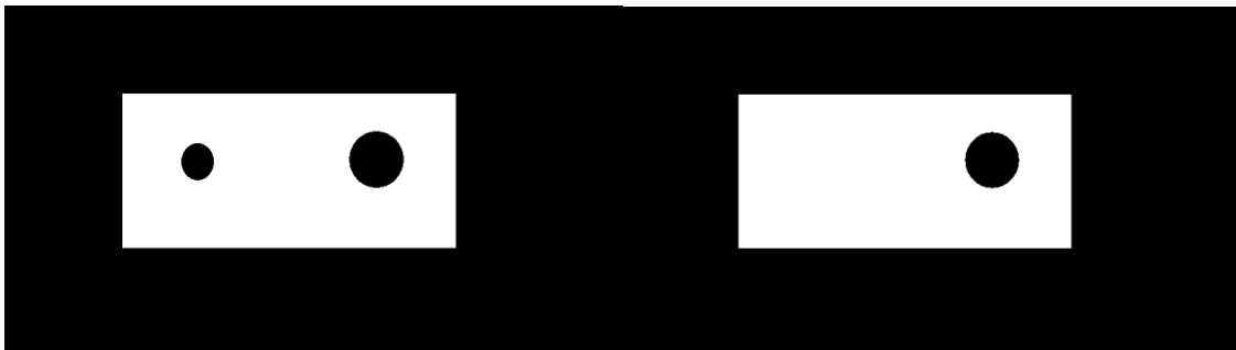
Figure 2.13 Left side of the image is original image; right side of the image is closed image.
