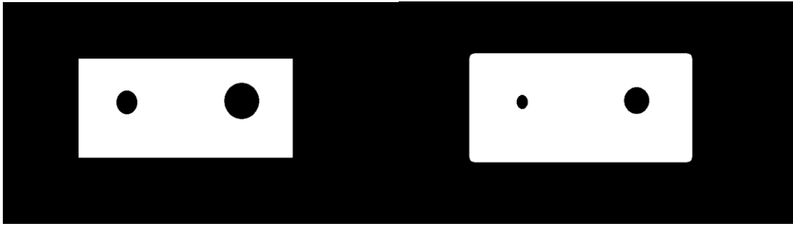
Figure 2.10 Left side of the image is original image; right side of the image is dilated image with certain disk structuring element.
