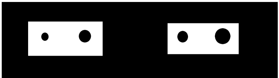
Figure 2.11 Left side of the image is original image; right side of the image is eroded image with certain disk structuring element.
