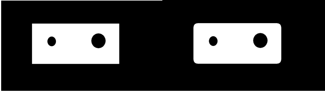
Figure 2.12 Left side of the image is original image; right side of the image is opened image.
