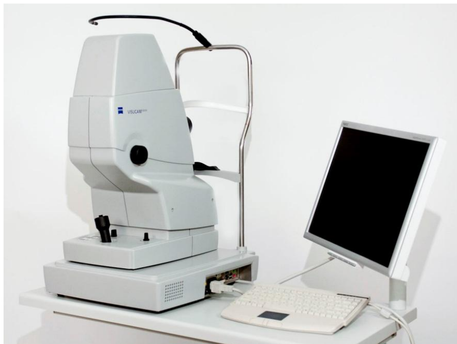
Figure 2.6 Zeiss Visucam PRO fundus camera is used in this publicly available dataset [30].
