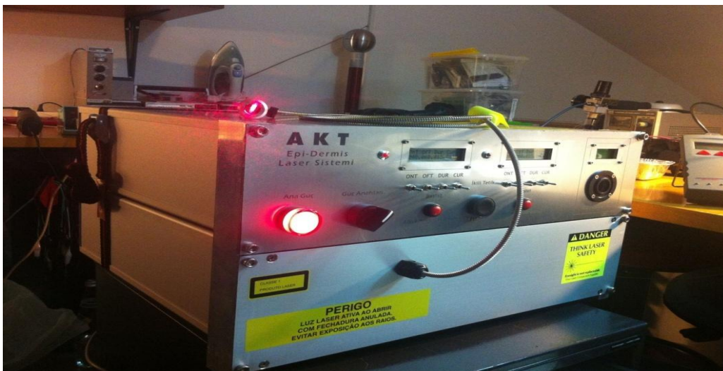
Figure 3.2 Completed AKT Dual wavelength Laser System
