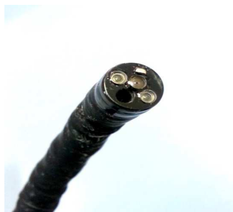
Figure 2.3 Endoscope Tip Part-Light, Air and Water Suction
