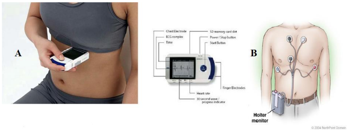
Figure 1.1 A. Portable ECG and B. Holter monitoring devices [4].
