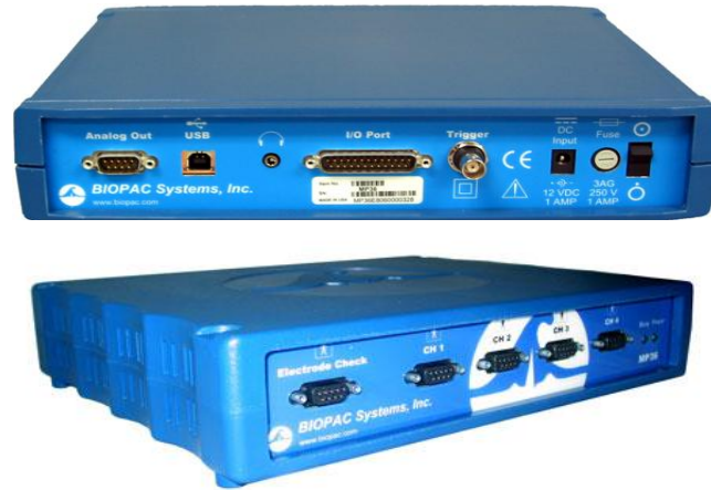
Figure 2.8 : EMG signal conducted by Biopac sys. MP 36 unit
