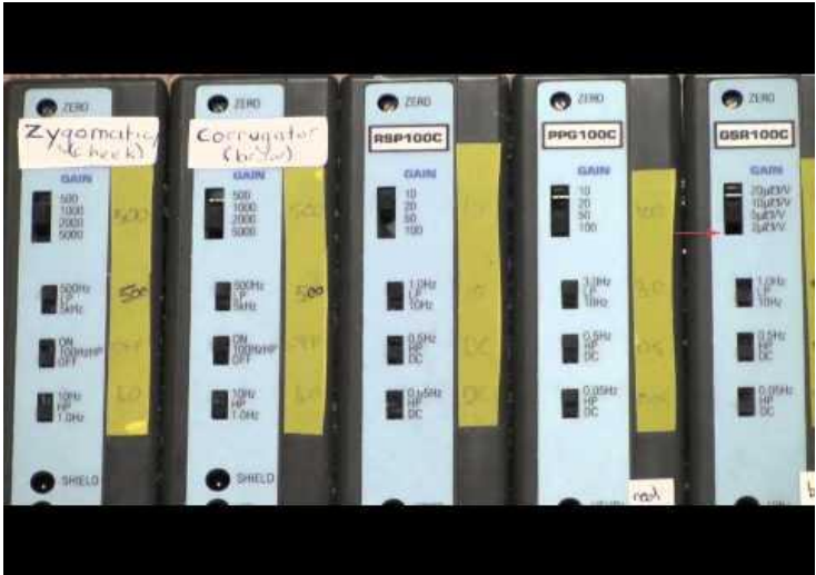
Figure 3.3 b) Galvanic Skin Response Amplifier GSR100C[44]
