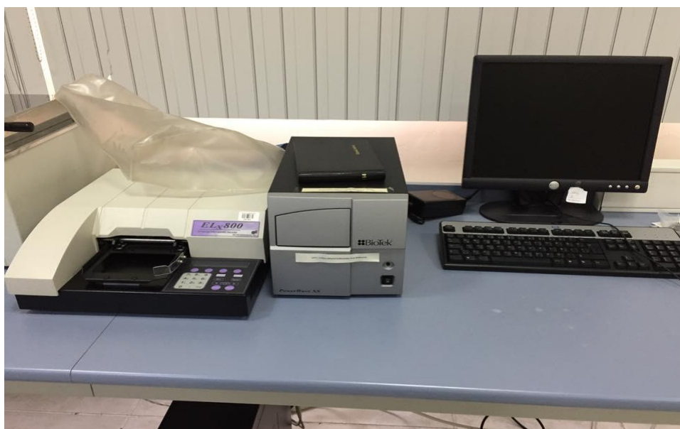
Figure 3.5 ELISA system ( microplate reader, power supplier and computer system)
