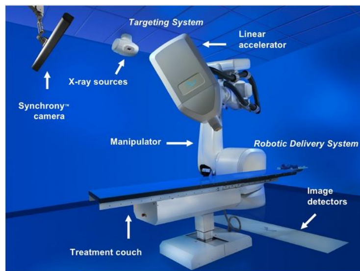
Figure 5.18 A modern Cyber Knife unit inclusive LINAC radiation delivery device ( http://www.slideshare.net/fovak/cyber-knife?next_slideshow=1 ) Date of access 11.01.2015
