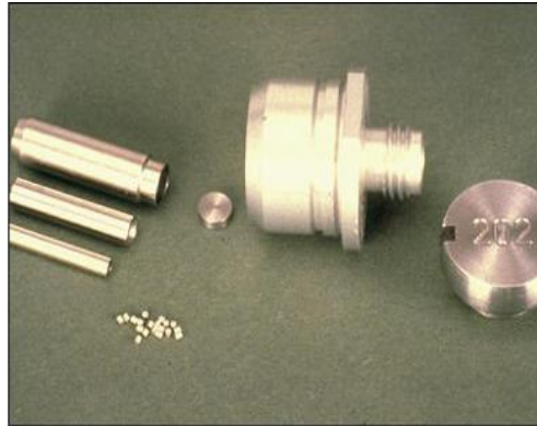
Figure 5.15 Cobalt 60 Radiation source for the Gamma knife ( http://www.lowback-pain.com/gammaknife.htm ) Date of access 15.12.2014
