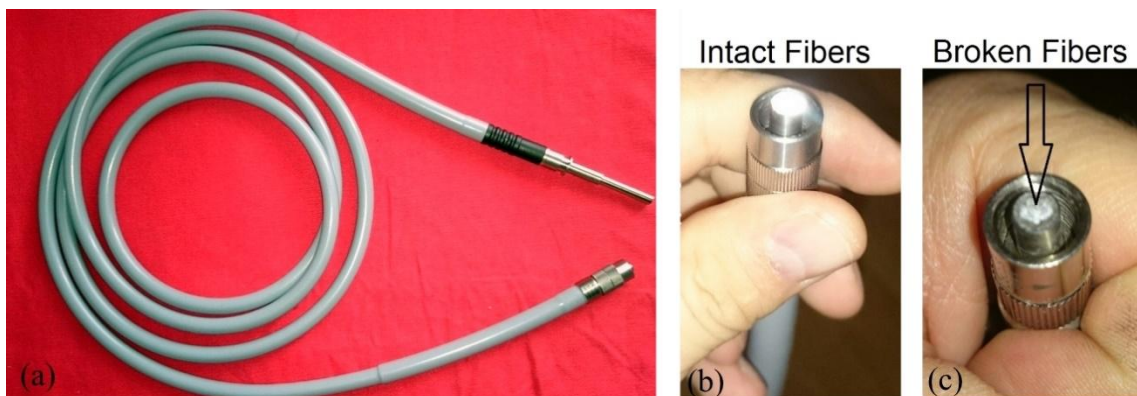
Figure 2.9 Fiber light cable (a) L:180cm, \Theta : 5mm (b) Intact fibers (c) Broken fibers
