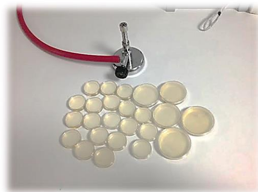
Figure 3.12 Cell culture dishes that are filled liquid TSA culture medium nearby bunsen burner
