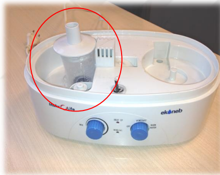
Figure 3.19 Modified nebulizer to calculate elapsed time for hydrogen peroxide consumption
