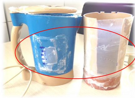
Figure 3.21 Modified heating coil to calculate elapsed time for hydrogen peroxide consumption
