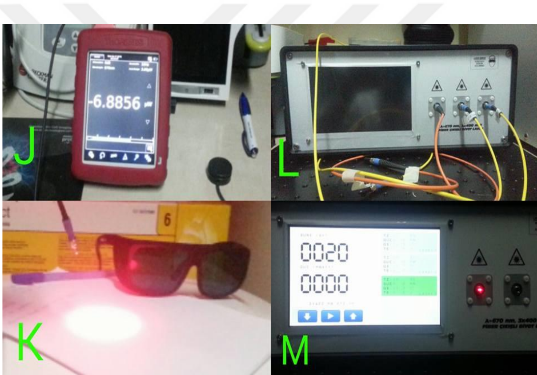
Figure 4.3: Laser System: J: Power Meter, K: Laser Beam & Eye protector and L: Laser system with three 670 nm emitting fiber outputs. M: Laser parameters can be set on the touch-screen.
