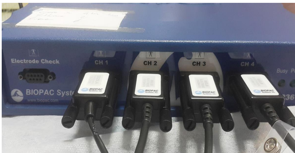
Figure 3.16 Channels of measurement cycle (CH 1.Hand dynamometer, CH 2.Extensors, CH 3. Flexors CH 4. Deltoid)
