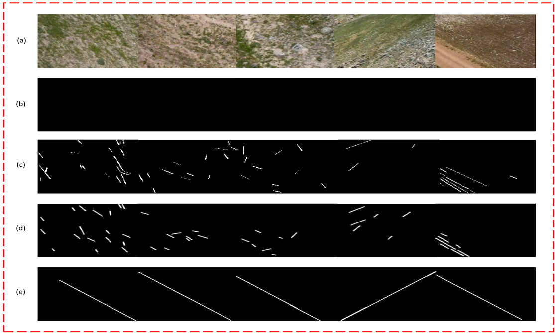
Figure 2.19. Edge/Line detection results: (a) VL images (without powerlines, correctly identified by our method), (b) Ground Truth of (a), (c) EDLines, (d) LSD and (e) HT. Edge/line detection methods incorrect.
