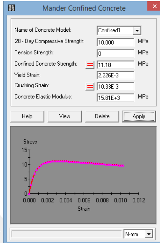
Figure 3.19 Confined concrete model of 75/40 substandard column
