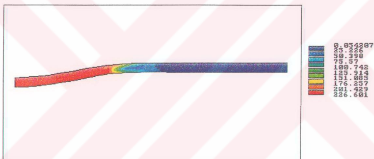
Figure 7.102. Equivalent stress contour on the longitudinal section of the circular cylinder with a hole ( a=18\text{mm} ) subjected to band pressure P=23\text{ MPa}
