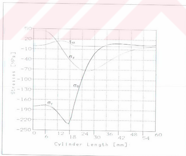
Figure 7.16. The stress components distributions through the length of the circular solid cylinder under band pressure P=220 MPa at r=0 (along symmetry axis of the cylinder)
