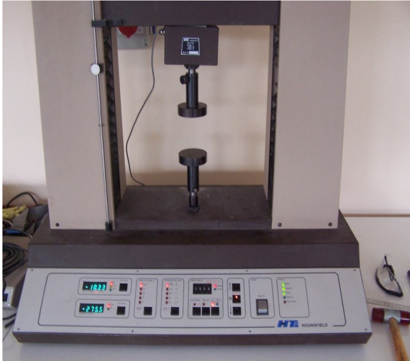
Resim 3.11: Çekme- Basma deney cihazı (HTI HOUNSFIELD® TEST EQUIPMENT LTD, REDHILL, ENGLAND ® )
