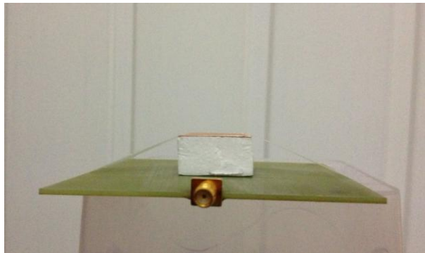
Figure 3.25 Side view of the fabricated patch antenna with the parasitic patch.
