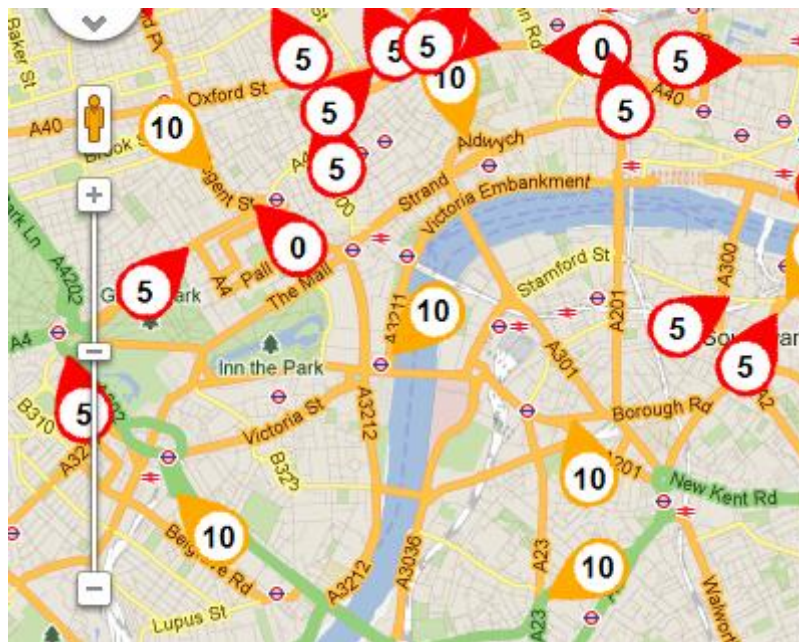
Figure 4.3: Traffic Master's live travel time estimation system that utilizes LPR
