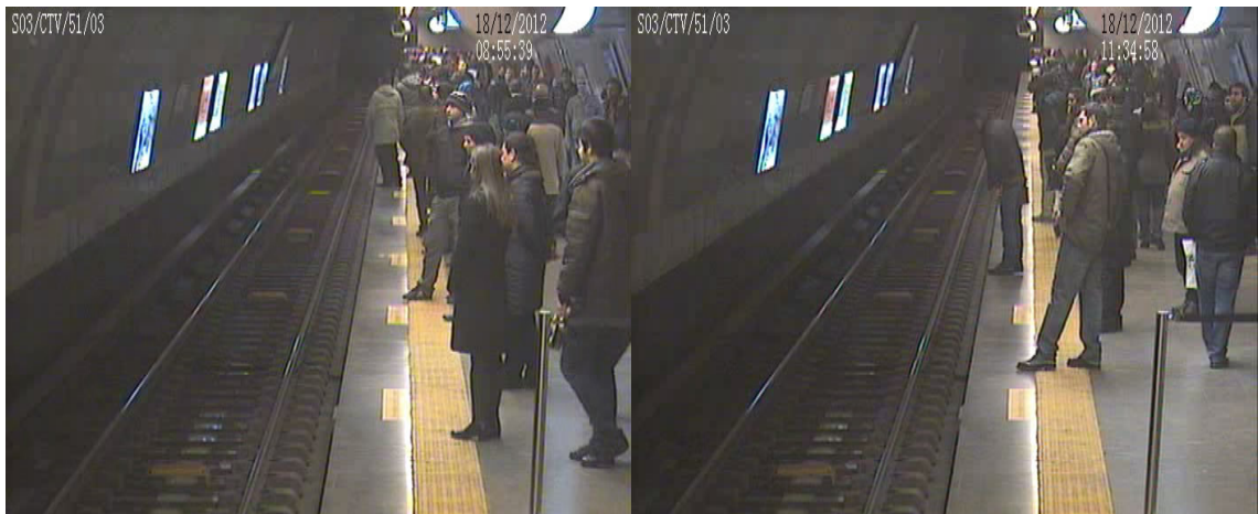
Figure 4.2: Sample images for SLI (security line intrusion)
