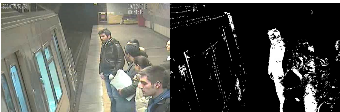
Figure 5.9: A crowded scene at the left and the foreground objects are at the right
