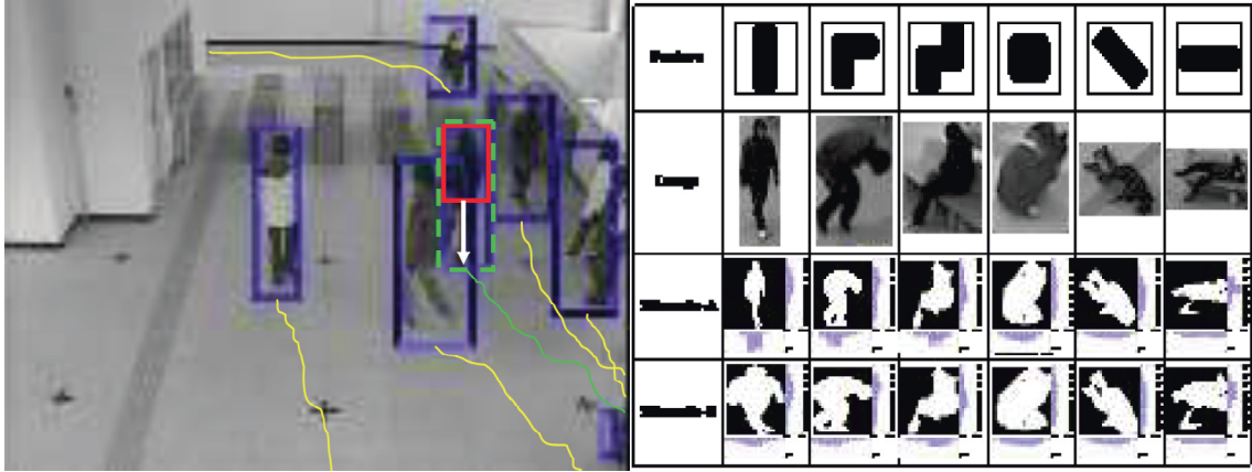
Figure 1.3: Tracking pedestrian locations on the left and posture recognition on the right
