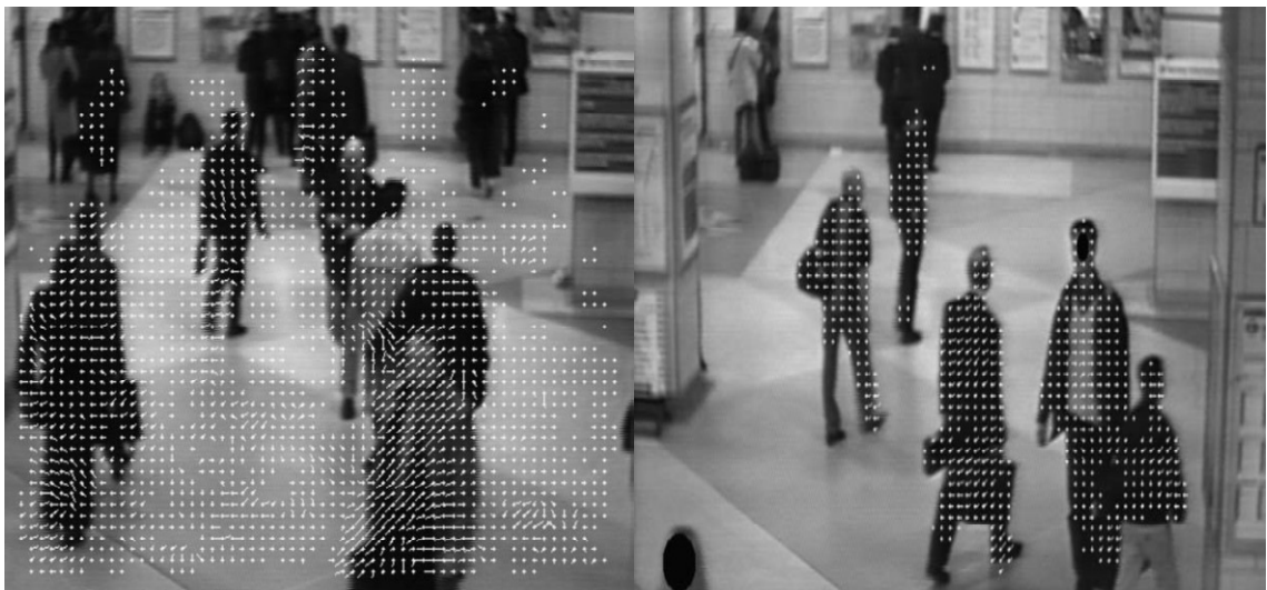
Figure 1.5: Sample image with raw motion vectors on the left and image with foreground filtered motion vectors on the right
