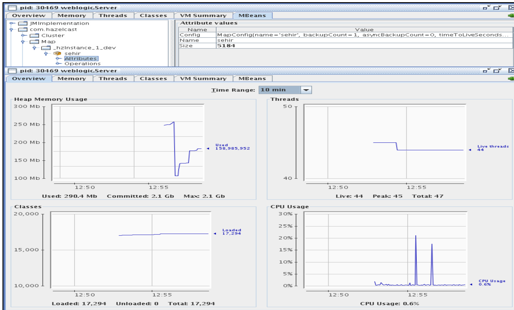
Figure 4.8: The results of CPU and memory usage in Hazelcast
