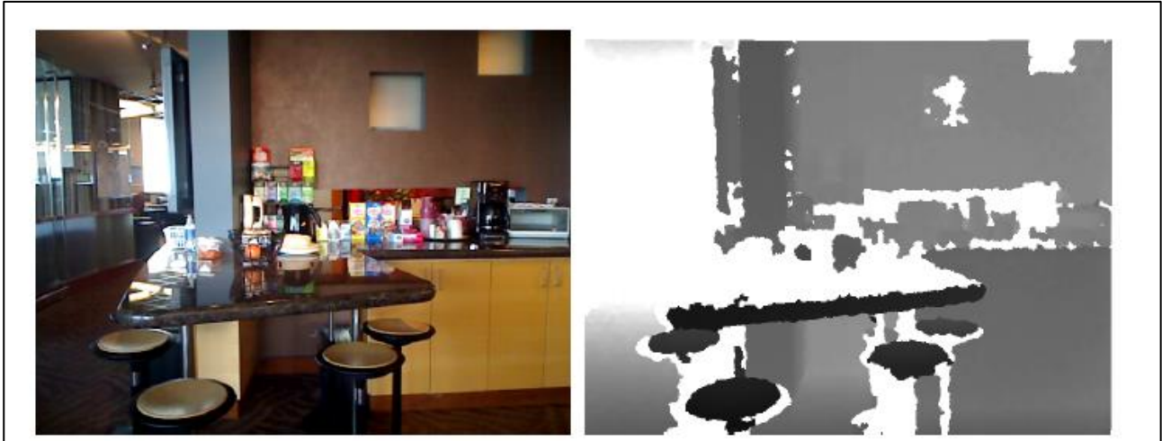
Figure 2.1 (left) RGB image and (right) depth information captured by an RGB-D camera. Recent systems can capture images at a resolution of up to 640x480 pixels at 30 frames per second. White pixels in the right image have no depth value, mostly due to occlusion, max distance, relative surface angle, or surface material. (Manuel Blum, Jost Tobias Springenberg, Jan Wulping and Martin Riedmiller, 2012)
