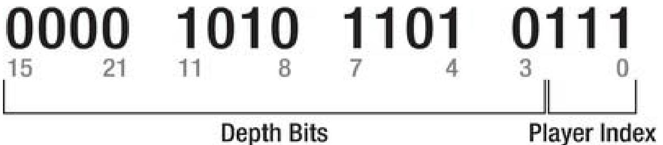
This means for a 640\*480 resolution frame kinect produces 16\*640\*480 bits. Also programmers can determine the player with mask 0000 0111.
