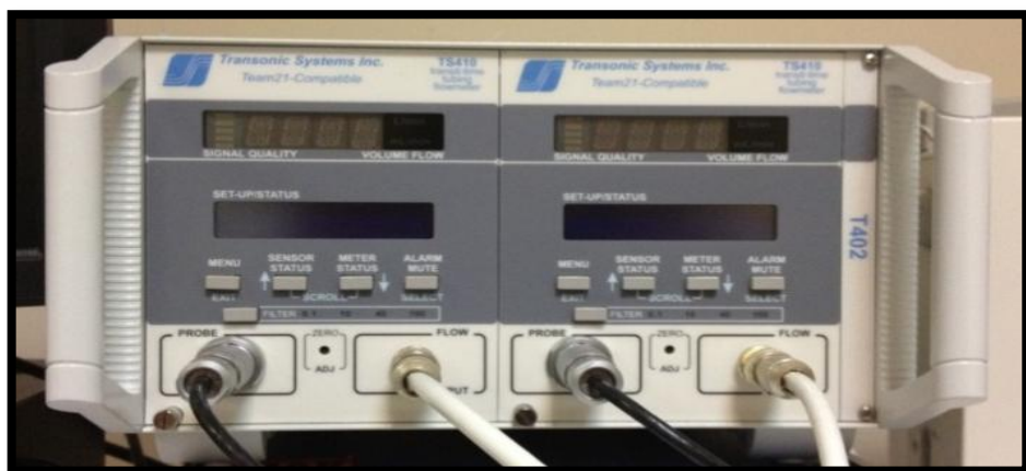
Figure 3.30: Transonic Systems TS410 Bypass Flow Meter Panel
