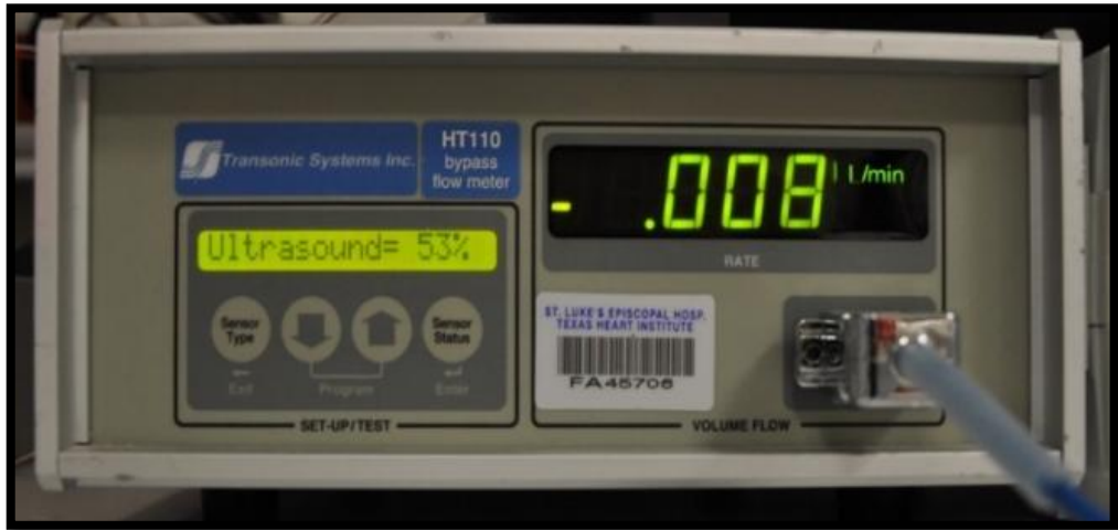
Figure 3.31: Transonic Systems HT110 Bypass Flow Meter Panel
