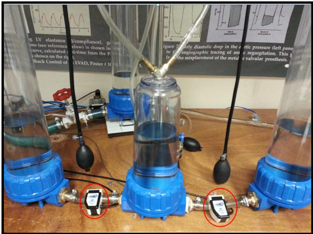
Figure 3.32: Transonic Systems Inc. Ultrasonic Flow Meter Sensor
