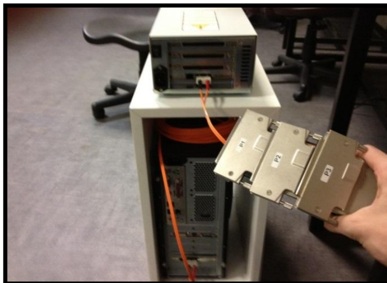
Figure 3.10: CLP1103 data transmitting cables
