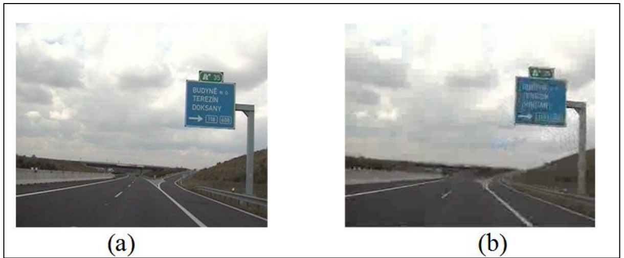
Figure 5.7: (a) Transmitted Common Intermediate Format (CIF) 352x288 MPEG-4 XviD (b) Received CIF 352x288 MPEG-4 XviD- PSNR: 29.13dB
