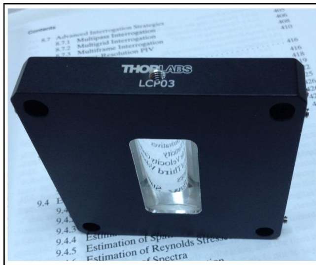
Figure 2.6: Light Sheet Forming Lens
