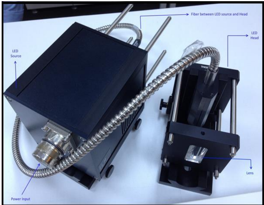
Figure 2.4: LED System and Head
