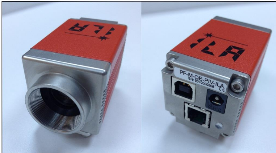
Figure 2.10: front and back view of Nano-camera
