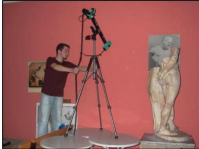
Figure 5.6: Using 3D Structured-Light Imaging System to Reconstruct the Weary Heracles Statue.
