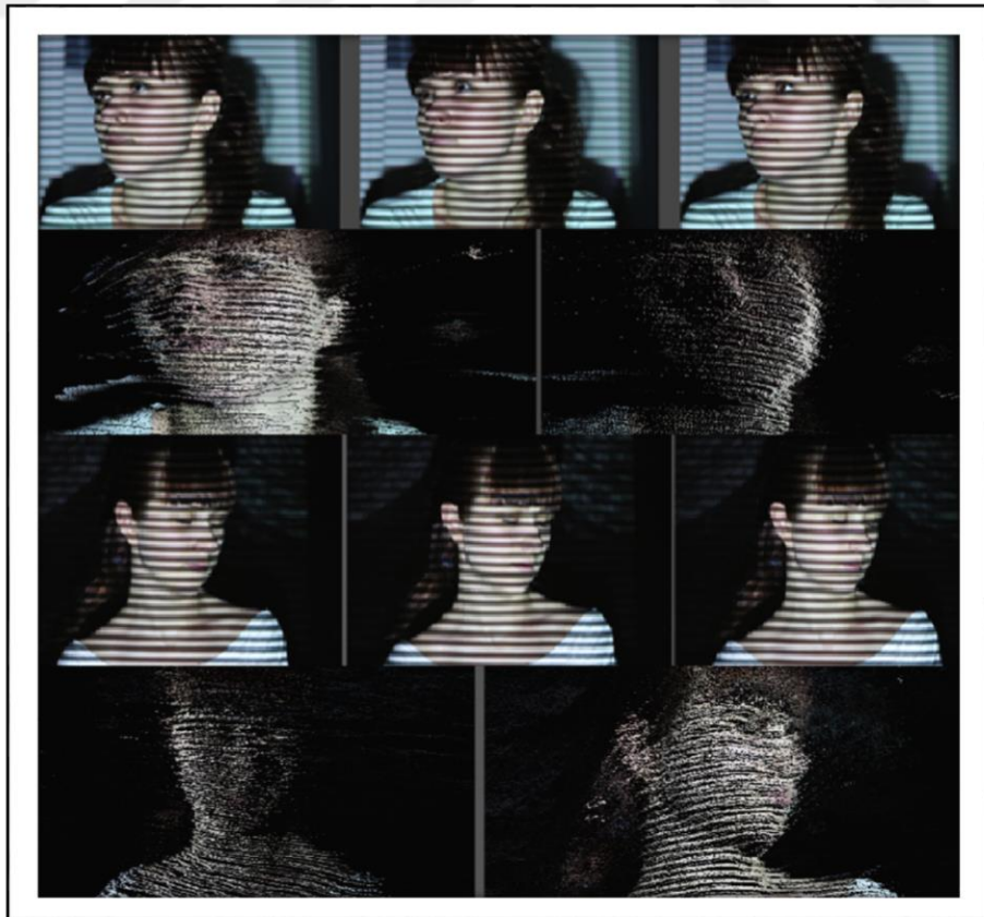
Figure 0.3: The Resulted 3D Images Captured By Using Phase Shifting Technique.
