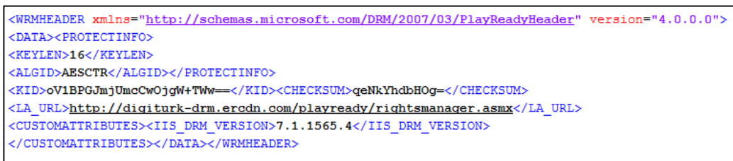
Figure 3.19: Decoded ProtectionHeader value
