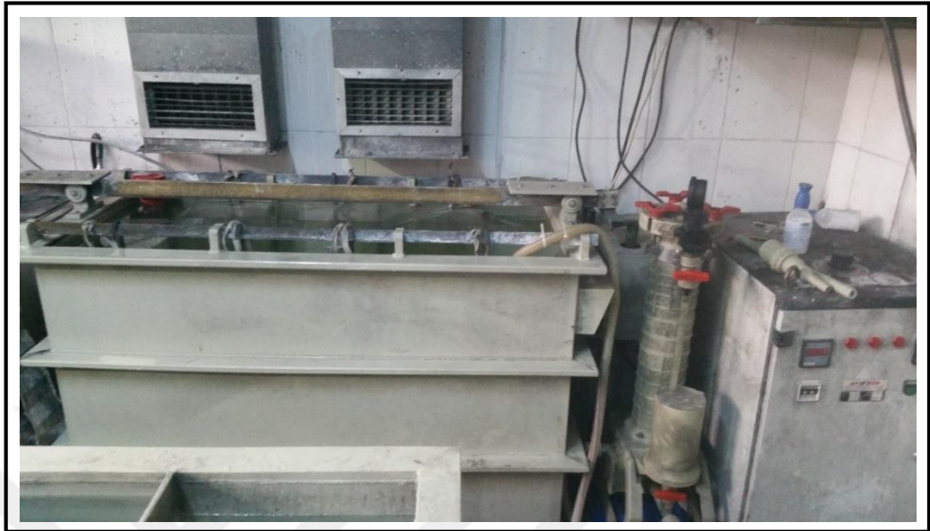
Figure 5.5: Cyanide Copper Bath and Electric Current that Temperature and Time Set
