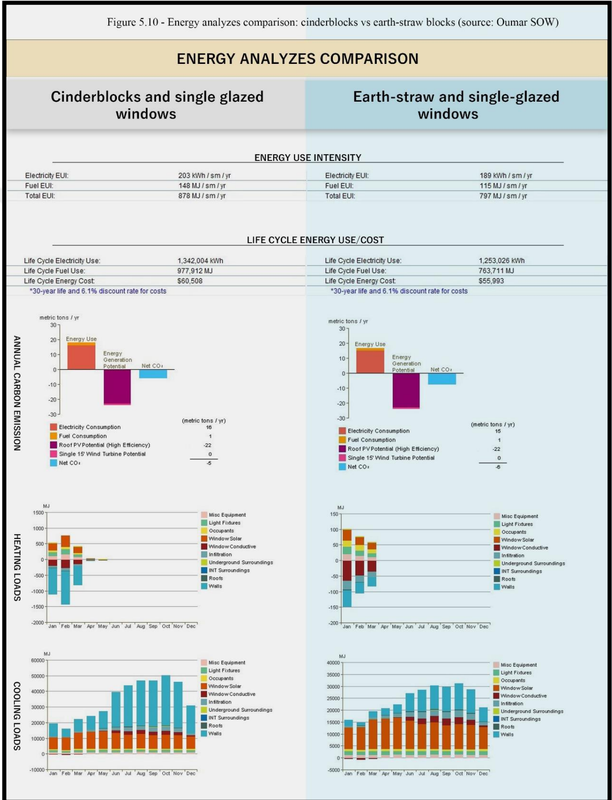
Figure 4.5: Energy analysis comparison of the same building with cinder blocks and earth-straw used as construction materials in Revit
