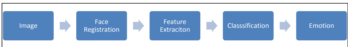
Figure 2.6: Basic structure of a facial expression recognition system.
