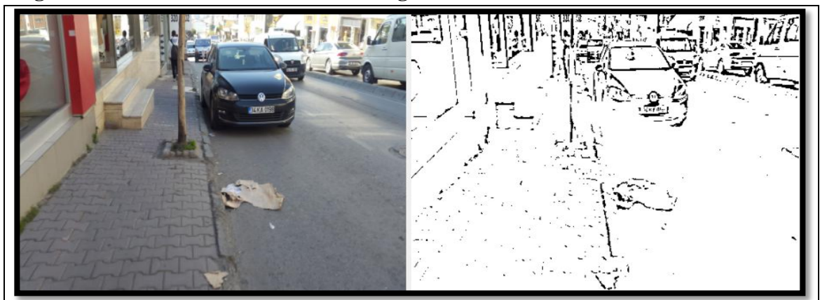
Figure 5.12: The binarization of the image contains a car far from the camera
