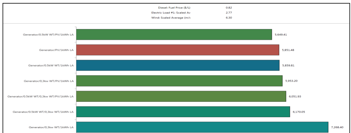
Figure 8.8: Graph of NPC of Load-shedding hour's optimal systems at 6.30m/s wind speed
