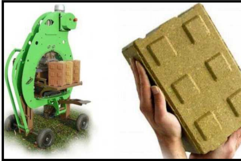
Figure 5.8: Mud Brick Hydraulic compressor
