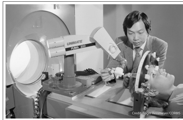
Figure 1.3: PUMA 200 holding a probe in brain biopsy procedure
