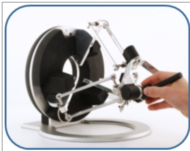
Figure 1.7: Omega.6; the master side of the surgical robotic platform.
