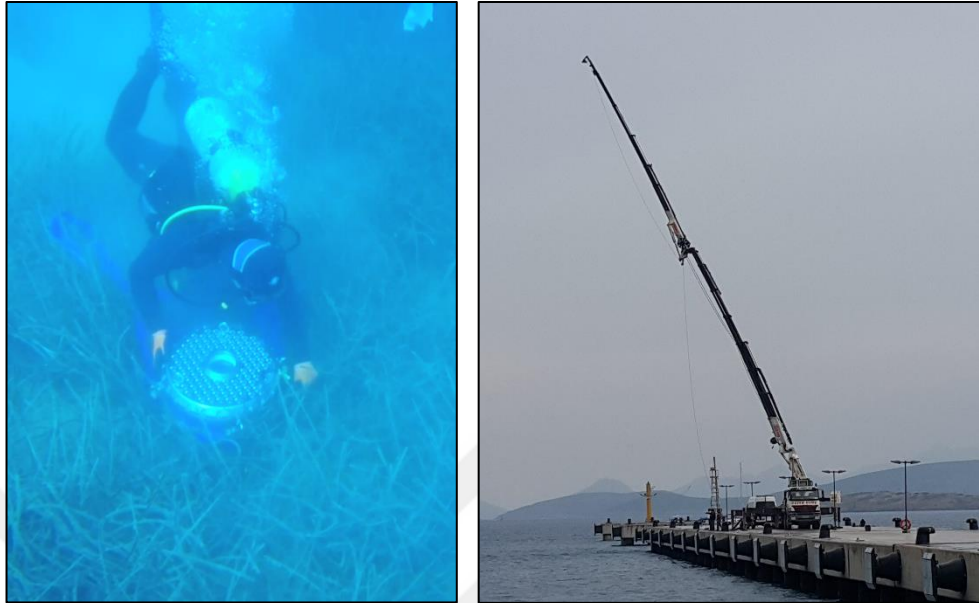
Figure 5.2: Underwater optical communication unit is placed on the sea floor and the free space optical communication unit is placed at the top of the crane.
