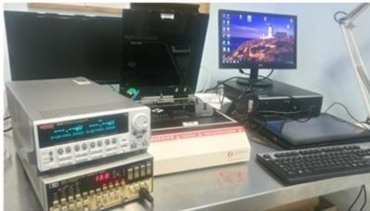
Figure 4.14. I-V measurement system
