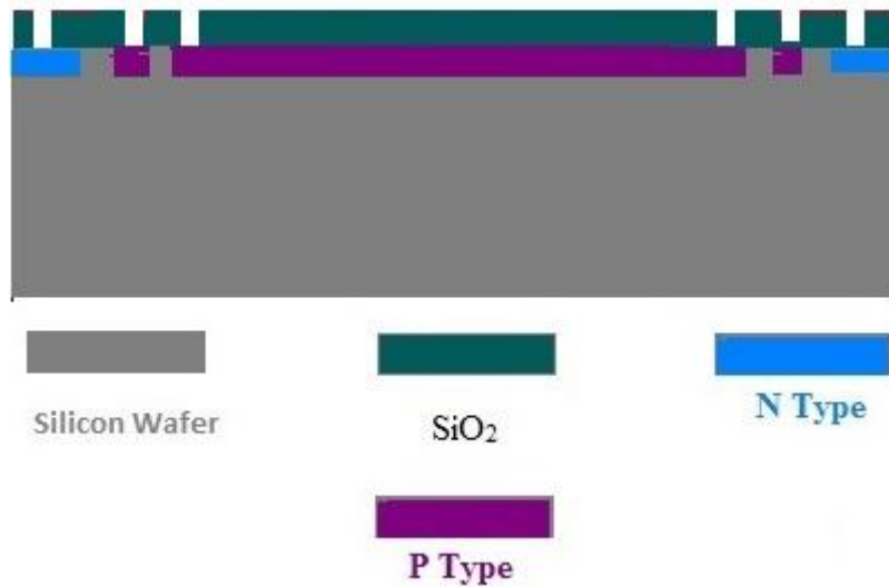
Figure 4.10. Wafer structure after liftoff process
