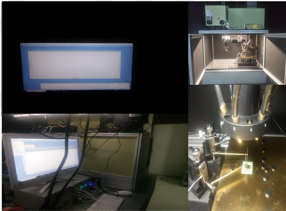
Figure 4.16. Spectral responsivity and quantum efficiency measurement system
