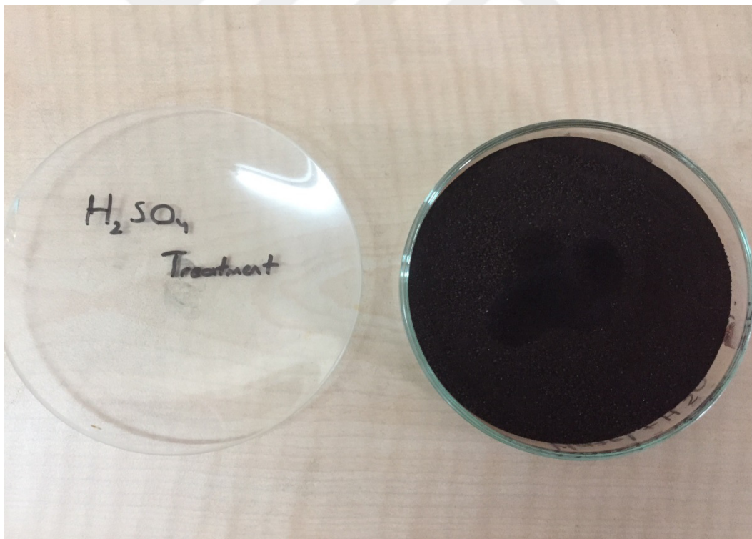
Figure 3.5. H 2 SO 4 treatment process nutshells
