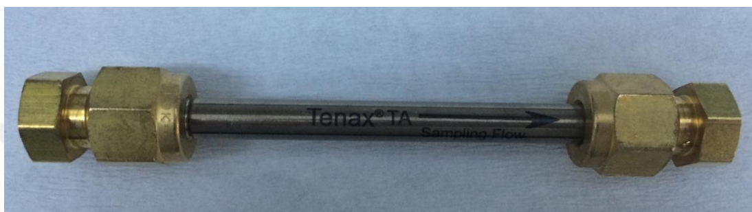
Figure 4.5. Tenax-TA tube used in passive sampling of Volatile Organic Compounds (Photo from our laboratory)
