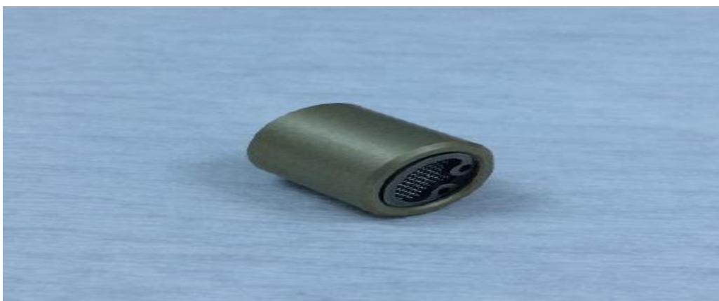
Figure 4.14. The diffusion head of Tenax-TA passive sampling tube (Photo from our laboratory)
