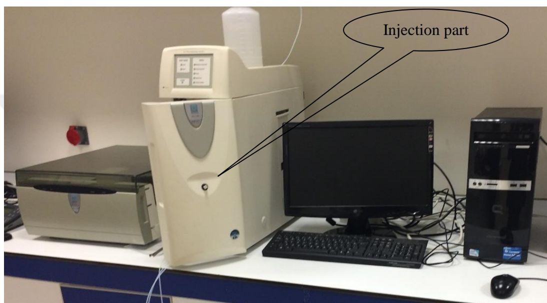
Figure 4.15. Ion Chromatography used in the analyses of inorganic components and injection part (Photo from our laboratory)
