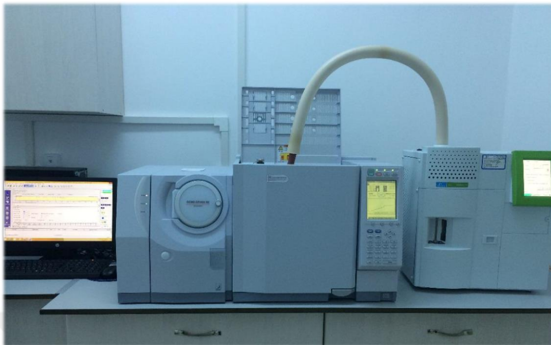
Figure 1.6. TD-GC-MS System using in the analyses of VOCs (Photo from our research laboratory)
