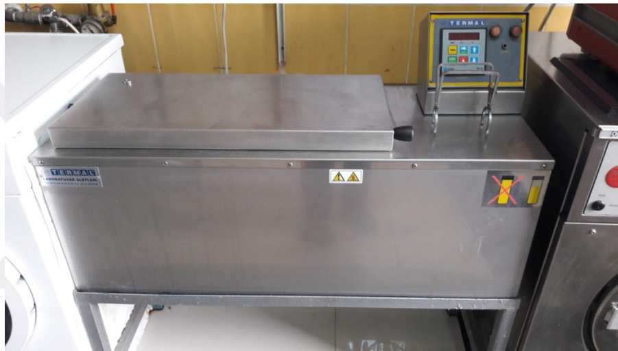
Figure 3.1. Mini high-temperature jet dyeing machine (TERMAL TM) used in dyeing process
