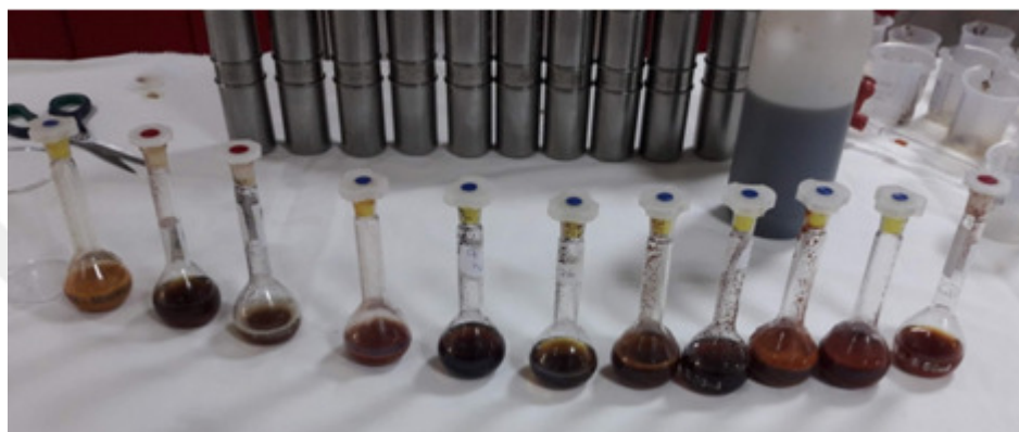
Figure 4.5. General appearance of disperse dye solutions (standard and nano dyes) and sample dyeing tubes
