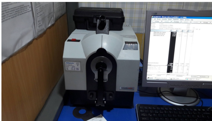
Figure 3.2. Datacolor SF 600 colour spectrophotometer for color control
