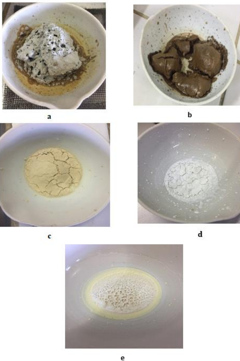
Figure 4.29. The images of Mg_{2.990}Ho_{0.010}B_2O_5 samples were synthesized with a) Gly, b) TA, c) CA, d) U, e) HMTA
