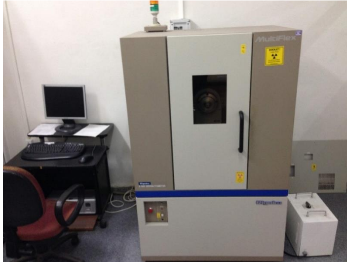
Figure 6.7. X-ray diffractometer for crystal structure analysis.
