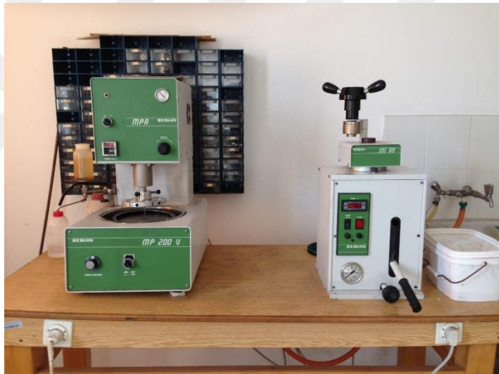
Figure 6.9. The polishing machine is on the left and the mounting press is on the right.
