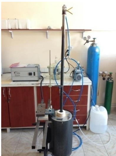
Figure 6.1. A vertical furnace and experimental set up for magnesium coating process.
