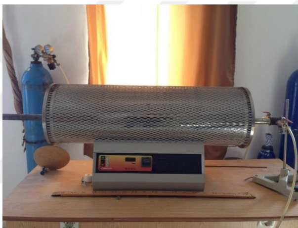
Figure 6.6. A programmable tube furnace with required installation parts.
