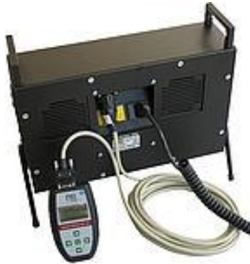
Şekil 3.16. MRU Air Fair Optrans 1600 is probu
