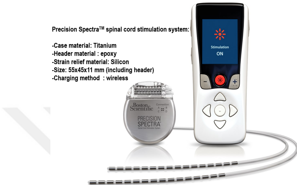
Figure B.1: Spinal cord stimulation system specifications (from https://www.bostonscientific.com/content/dam/Manuals/us/current-rev-en/91057051-01RevA_Precision_Spectra_IPG_DFU_en-US_S.pdf ).
