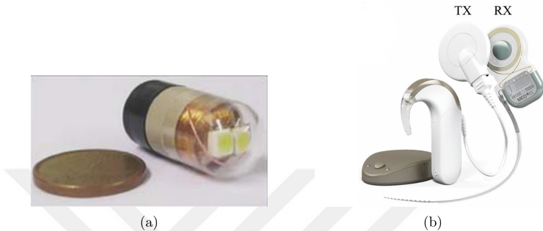
Figure 2.2: Examples of devices powered with RF waves: (a) an assembled receiver in bio-compatible package to be used as endoscope next to 1 eurocent coin, (b) cochlear implant, RX coil positioned beneath the skull behind the ear to be powered by the external coil TX [29, 31].
