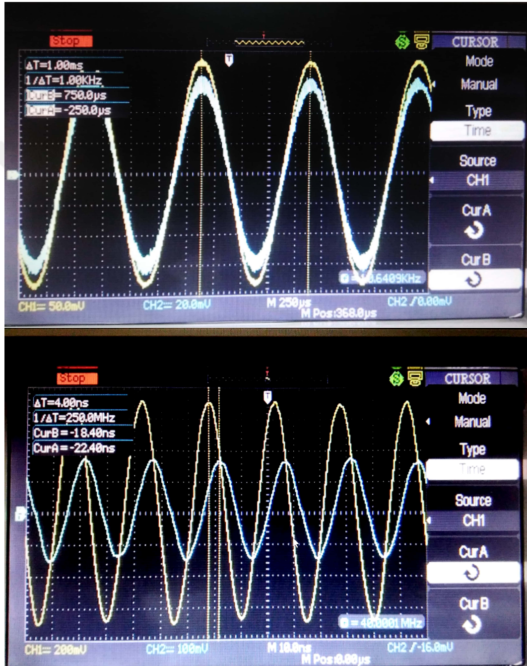
Figure 4.19: Stator voltage in yellow and R1 voltage in blue on the oscilloscope when applying a source signal at 1 KHz (top) and 40 MHz (bottom).
