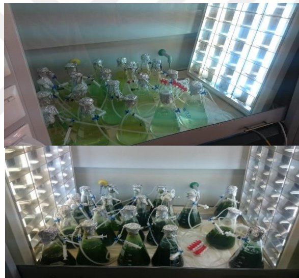
Figure 2.2. The cultivation of isolated microalgae for calibration curve withdrawal and elemental analysis
