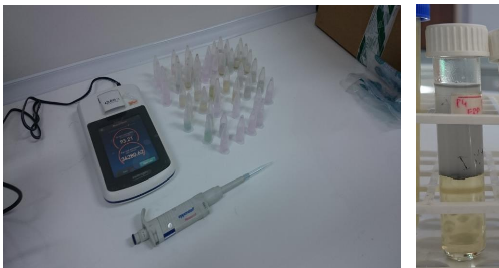
Figure A.16. Left: fluorometric method for lipid determination, Right: Separated two phase during lipid extraction
