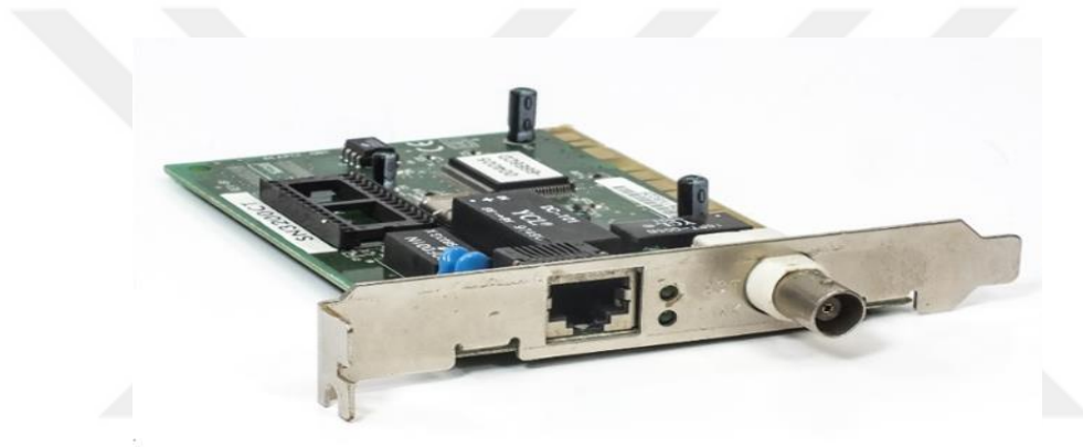
Figure 6.BNC connector (Bayonet Neill-Councilman Connector) [55]
