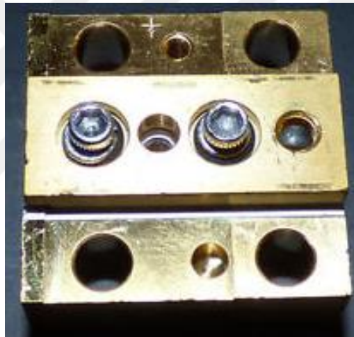
Figure 2.9: Traditional high-power Coherent Laser Diode Bar packages
