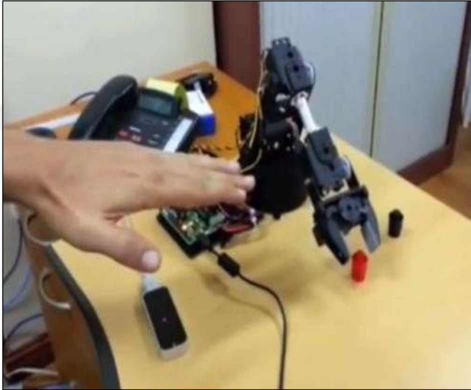
Figure 4.6: Robotic Arm Controlled With Leap Motion
