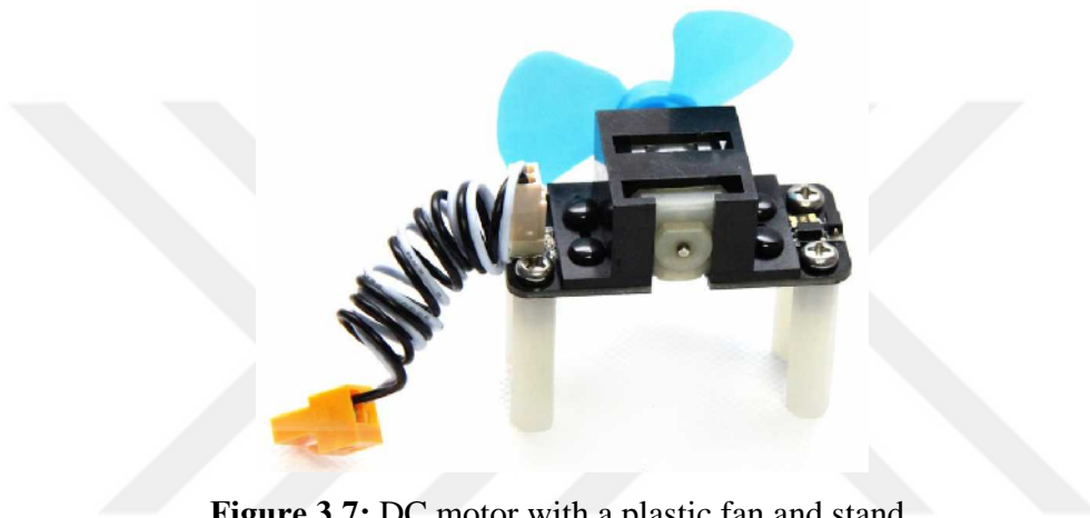
Figure 3.7: DC motor with a plastic fan and stand.
